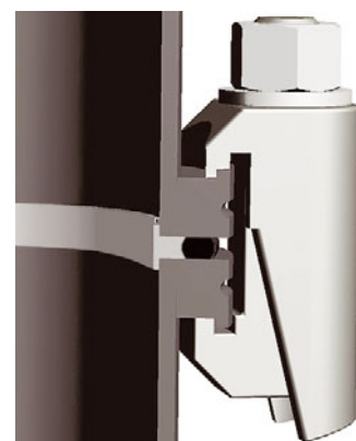
Figure 1: In case of ISO-KF and ISO-K up to DN 250 size, the centering ring is specified, so that the O-ring is compressed from about 5 mm to exactly 3.9 mm.
