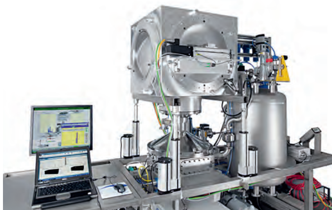
VAT particle test stand for particles > 10 nm
